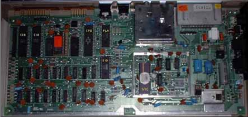
Abb. 7: Assy 250407 ca. aus 1983/ 84. PLA ne- ben CPU, SID darunter
